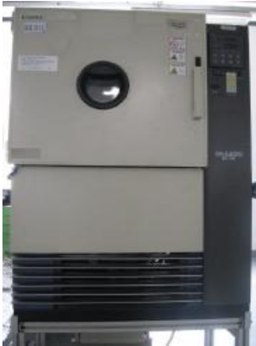
Temperature Chamber Range: -40°C ~ 100°C
