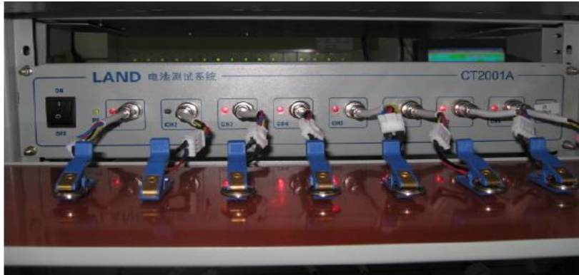
Small current cycler (5V/10mA) mainly for half cell testing
