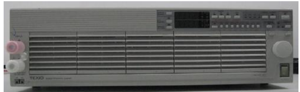
TEXIO electronic load (200V/200A) Programmable: can set CCD, CLD, CPD
